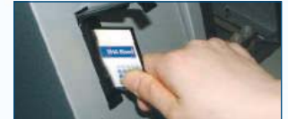
A: Insert an EZ1 Card containing the appropriate nucleic acid purification protocol.
